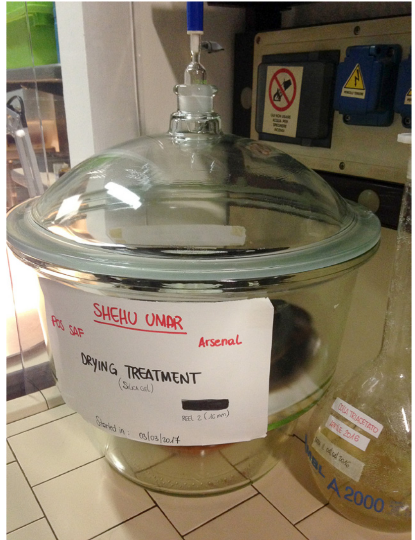
Dehydration treatment of a 16mm positive reel affected by the vinegar syndrome
